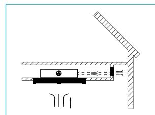
**!** In this version the check valve must not be assembled: remove it if it is on the air outlet fitting of the motor.
